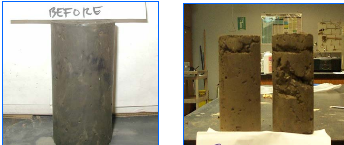
Figure 6. Left photo of a properly prepared test cylinder. Right photo of a poorly prepared cylinder that will result in poor test results for strength and permeability.
