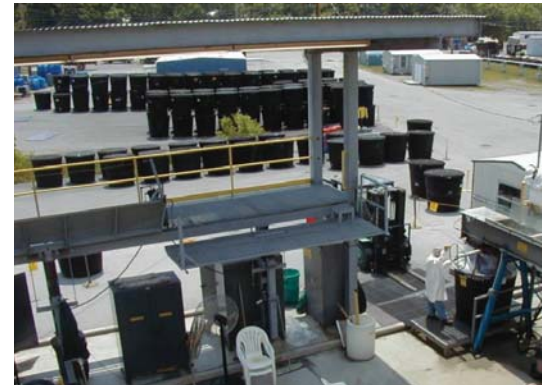
Blended solids being loaded into 21st Century containers and prepared for shipment.
