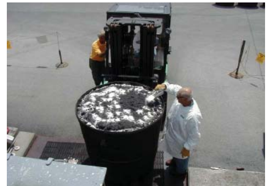
Quik-Solid® granular media being applied to top layer of solids prior to shipment to prevent free liquids from condensation and solids compression.
