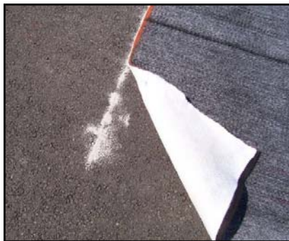
The Reactive Core Mat is filled with Organoclay, which is used to adsorb contaminants.
